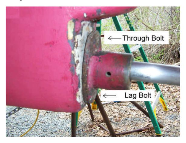
With a little patience and a little twisting and prying, the shaft log loosened from the hose and slid out. Once I knew it was coming out, I cleaned and polished the prop shaft and then removed the shaft log. The hull was then sanded and cleaned in preparation for putting the shaft log back. I made sure I had plenty of polysulfide sealant to re bed the shaft.
