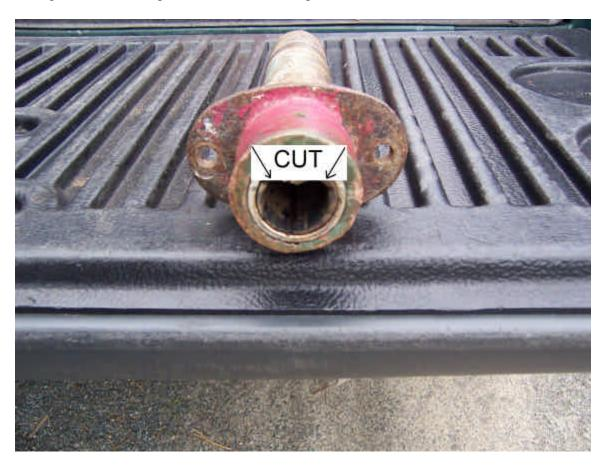
After cutting was completed, I tried to tighten the set screw all the way all the way through opening up the cutless bearing where it was cut. But that trick never works, so I removed the set screw, inserted a punch into the hole and beat it with a hammer.
