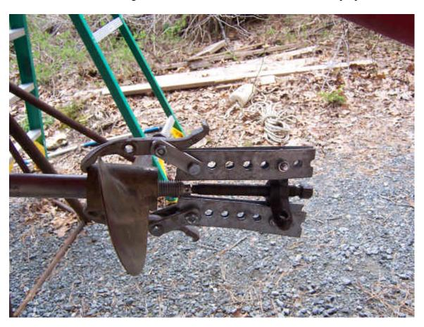
I made sure the jaws were centered, the threaded rod was centered on the shaft, and then using a socket wrench tightened the threaded rod on the shaft. After a few turns and a few taps with a plastic mallet, the prop came off. I usually take my props off every year just because that makes it that much easier the next time. There is nothing worse than trying to get a prop off that has been on a few years.
