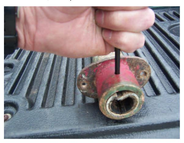
Once the bearing was split, the pressure was released from the wall of the shaft log. Now I could move to the next step and push the bearing out. I used a piece of 1 inch I.D. black gas pipe which is just the right size to fit in the shaft log and still catch the bearing on the inside. I then smacked the pipe a few times and the bearing came out.
