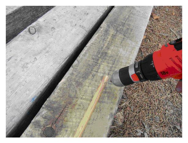
After completing the drilling, I turned each piece over and counter sunk each hole on the back. The next step is to carefully tap the nails though the holes all the way until the heads are countersunk. Apply ½ inch double sided foam tape to the back of each thus insulating the nail heads from the spreader.
