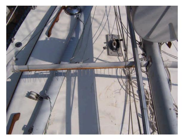
With the mast up, they shouldn't be too noticeable and the thin profile will keep the sails from catching on them. I made a small piece for the masthead while I was at it. The cost of making these was about six bucks for the nails and I had everything else on hand. The total time to build them was one hour, not including letting the varnish dry.
