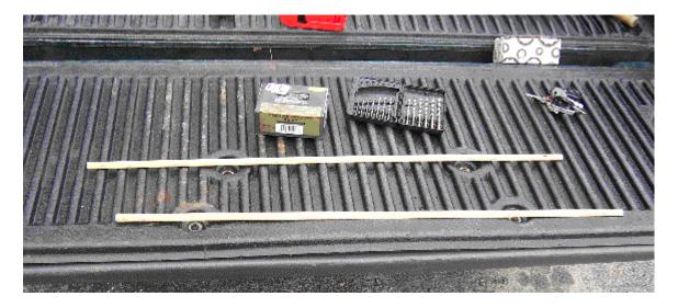
Next, I laid out marks every inch along, and marked the center line along each piece. I then drilled holes at each mark alternating between vertical and about 40 degrees from vertical. I think a drill press would come in real handy here, but I don't own one so I used a protractor and drilled by hand.
