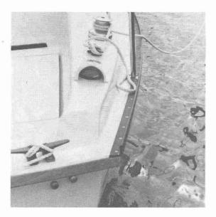
The Watkins 32 is built to last. The hull is heavily built of solid hand laid-up fiberglass to provide years of service. Watkins has avoided foam and balsa cores due to the potential for delamination and water absorption. The rigging is oversized again to provide an extra degree of reliability.
