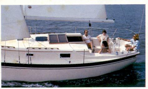
The Watkins 32 is a superb sailer in both light and heavy seas. The efficient hull cuts thru the water with a small bow wave and a clean wake. With a ballast ratio of approximately 50%, the boat is stiff as the wind picks up, yet her hull lines allow a slight heel in light air.
