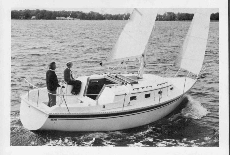
The Watkins 29 is an exceptionally strong boat with a hull constructed of solid hand laid-up fiberglass. Watkins uses a cored construction in the deck for lightweight stiffness but never in the hull. Mast, rigging, lifelines are all "next size up" for reliability.
