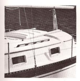
The Watkins 25 is built to last. The hull is heavily built of solid hand laid-up fiberglass to provide years of service. Watkins has avoided foam and balsa cores due to the potential for delamination and water absorption. The rigging is oversized to provide an extra degree of reliability.
