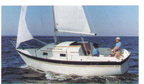
The Watkins 25 was designed to meet the need for a roomy trailerable boat. The maximum beam is 8 feet yet the interior space below is exceptional. The 25 has excellent sailing qualities with fairly deep "V" sections forward and a flat run aft. The fixed keel with internal ballast eliminates the many problems associated with swing keels or center boards.
